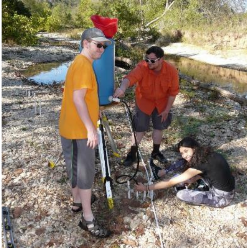
UofM Civil Engineering undergraduate students Spencer Drum, Justin Lawrence, and Carla Meier (left to right), measuring hydraulic conductivity within a river gravel bar on a research site at Bull Creek, Missouri Ozarks.
